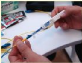
How to clean an LC connector with a pen-style click cleaner
