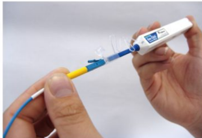
How to clean an LC connector with a pen-style click cleaner
